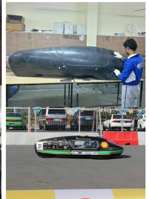
5) Carbon fiber Car shell for Shell Eco Marathon 2015:
