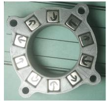
Stator six Poles viewing using magnetic film:
