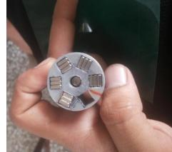
Rotor four Poles viewing using magnetic film:
