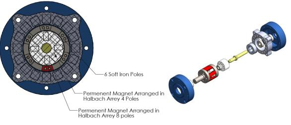
Prototype 1 of Magnetic gearbox for proof of concept:
