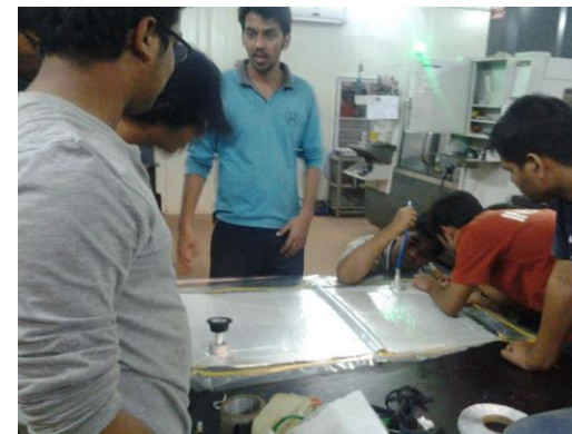
4) Vacuum bagging for the final Carbon fiber part:
