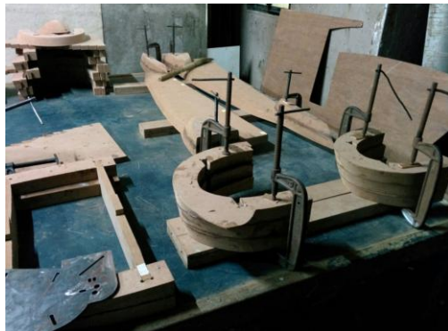
1) Pattern Machining from MDF:
