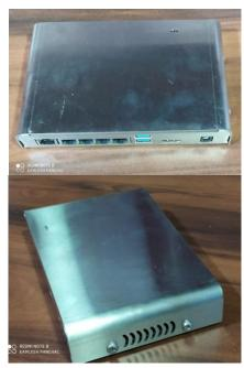
Mini Solar Module EL testing Enclosure.
