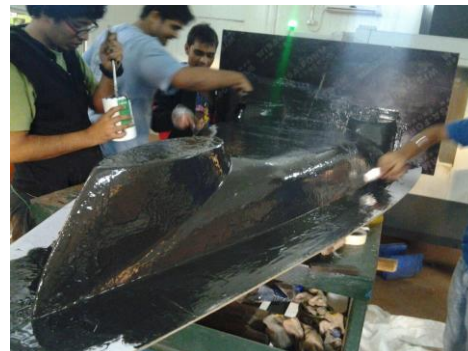
3) Glass fiber Mold Making:
