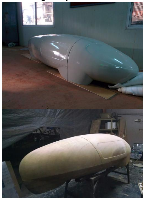
2) Fixing patten parts and finishing the pattern:
