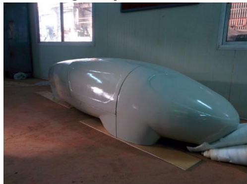
2) Fixing patten parts and finishing the pattern:
