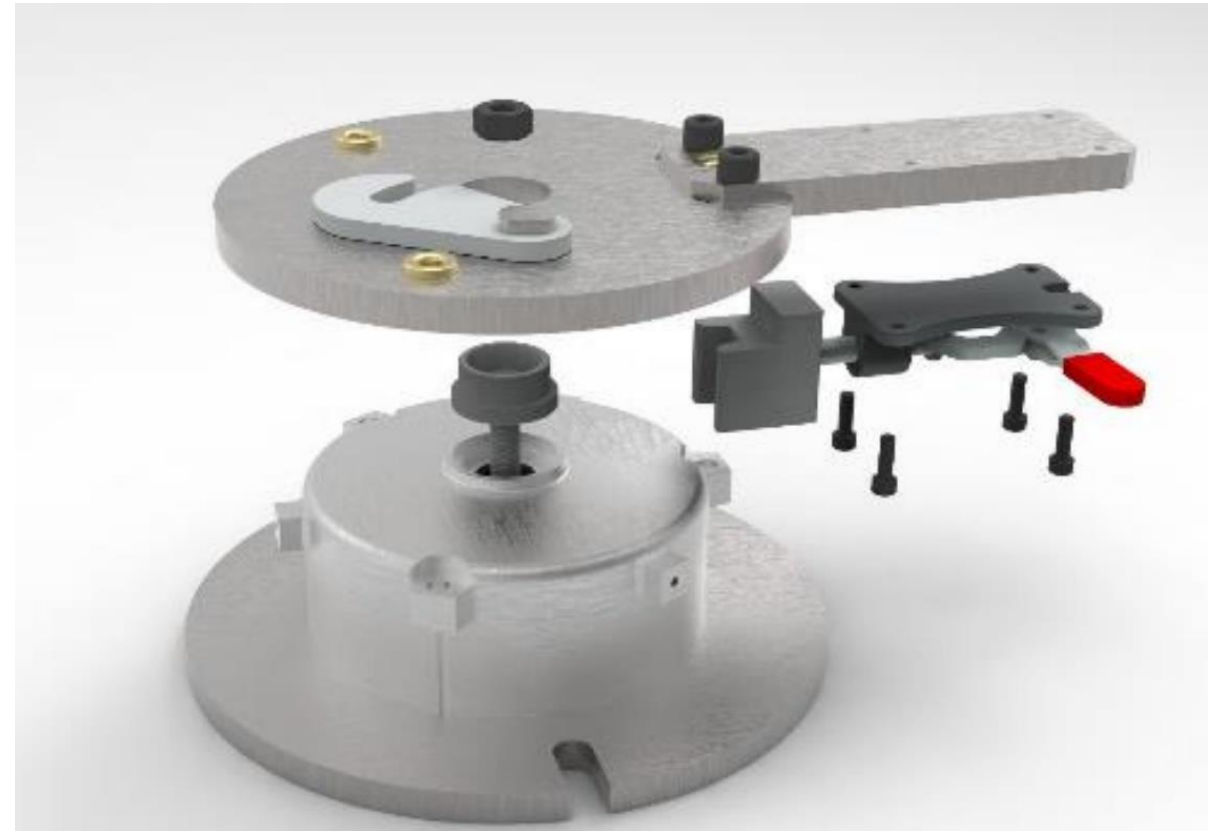
Exploded view drill jig station 1 :
